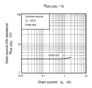
Drain-source ON resistance RDS (ON)  $(\Omega)$
